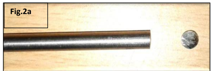
Figure 2a: Grade 5 Titanium rods sectioned into discs of identical dimensions.
