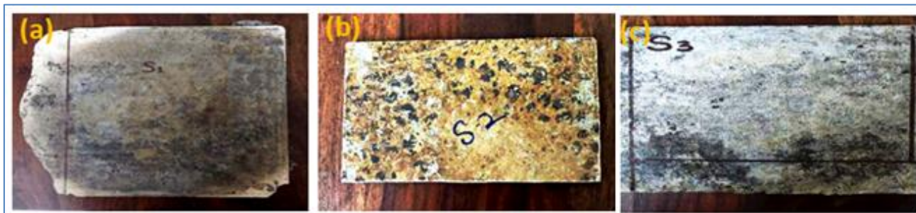
Figure 2: (a) PBC 1 (90% PEEK, 10% Basalt fiber); (b) PBC 2 (80% PEEK, 20% Basalt fiber); (c) PBC 3 (70% PEEK, 30% Basalt fiber)
