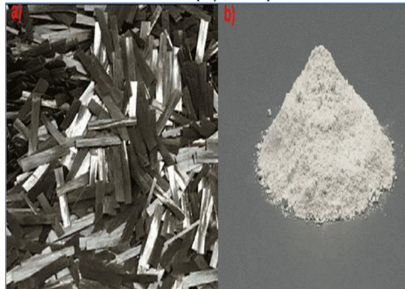
Figure 1: (a) Chopped Basalt fiber and (b) PEEK matrix (Powder)
