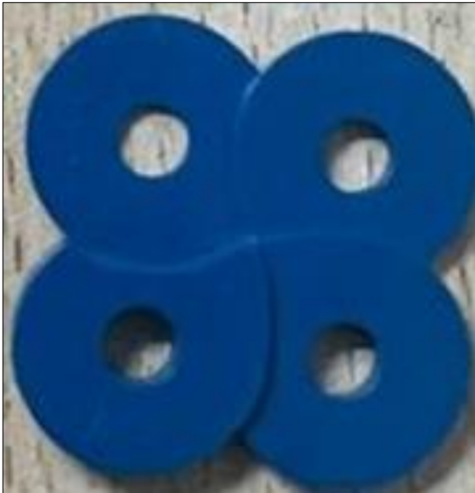
Figure 1: Disc specimens 10 mm in diameter x 1.5mm in height dispensed in disposable silicon molds in the form of round discs.
